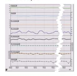
A control chart helps with the quality evaluation of the process. The normal distribution with the calculated parameters in the selected periods per channel reveals the quality status and the regulatory compliance.
