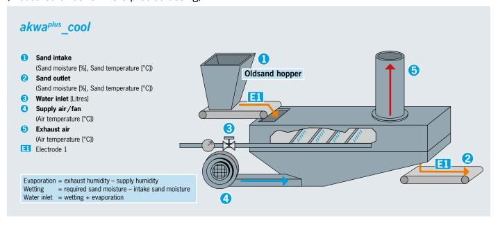
**The task:** Assuring the quality of the moulding sand starts with the cooler. Its balanced moisture output facilitates the mixer's work, as the mixer is not able to balance everything out. An additional measuring device, coupled with a controller, is intended to significantly reduce fluctuations in the output moisture. **The used sand should be evenly cooled and evenly moistened.**
